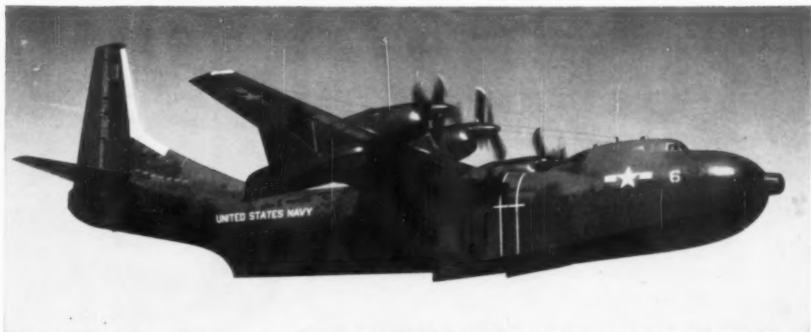
R3Y-1 TRADEWIND is powered by four Allison T40 turboprops rated at 5,500 eshp. Overall length is 142.5 ft., wingspan 145 ft.
